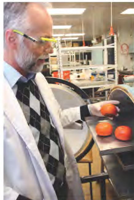
Persimmons are placed in a vacuum chamber to investigate induction of disease resistance through the application of a mild hypobaric stress. In 2011 persimmons were worth $7 million in annual export value to New Zealand. They can be stored for three or four months.
