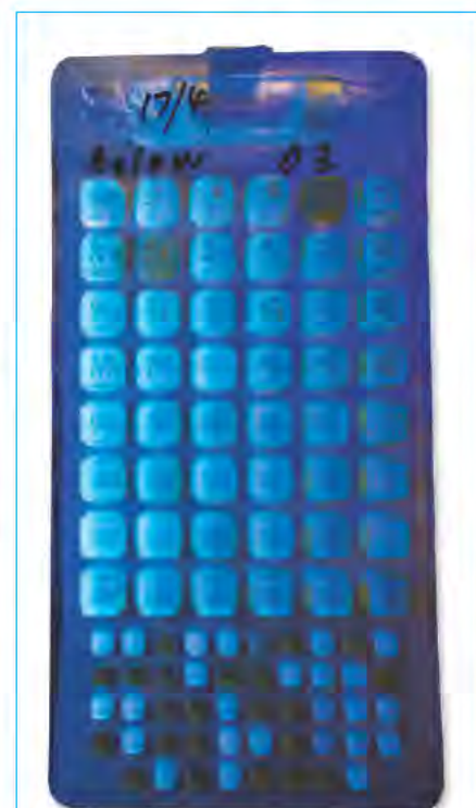
A 96-well tray filled with a roof water sample and test reagent after incubation. Forty-seven large wells and 24 small wells fluoresce under UV light and result in an Escherichia coli count of 270 organisms per 100 millilitres.
